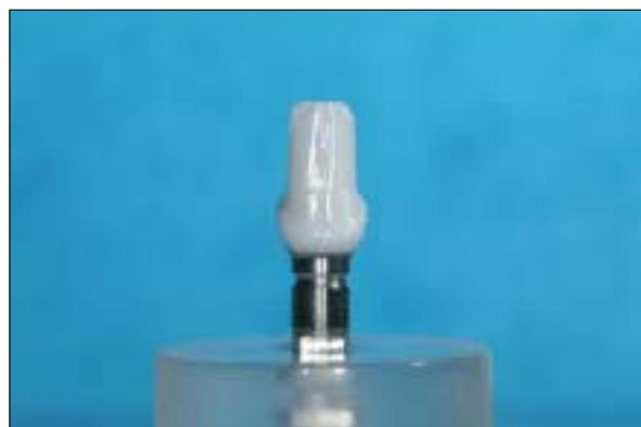
**Fig 4** Testing apparatus. The abutment was prepared with diamond burs to achieve a shape comparable to that of an average-sized maxillary central incisor aligned with the long axis of the implant.
