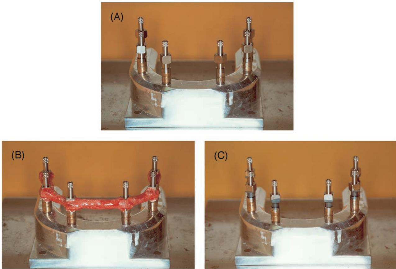
**Fig. 3.** **A**, Non-modified square impression copings (group 1). **B**, Nonmodified square impression copings rigidly splinted with acrylic resin prior to impression procedure (group 2). **C**, Square impression copings previously airborne particle-abraded and coated with impression adhesive (group 3).
