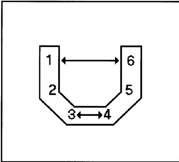
**Fig. 2.** Schematic representation of metal model. Implants and abutments were numbered 1 to 6. Distance between most posterior abutments (1 and 6) was 50.428 mm and between most anterior abutments (3 and 4) was 20.878 mm.
