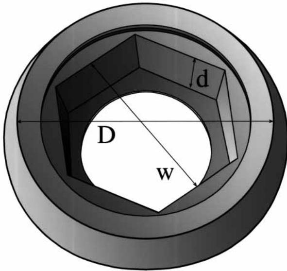
**Fig. 1.** Schematic representation of implant-abutment contact surface of UCLA abutment illustrating 3 parameters examined in study: depth ( $d$ ) of internal hexagon, flat-to-flat dimension ( $w$ ) for opposing surfaces of hexagon, and apical diameter ( $D$ ) of abutment.
