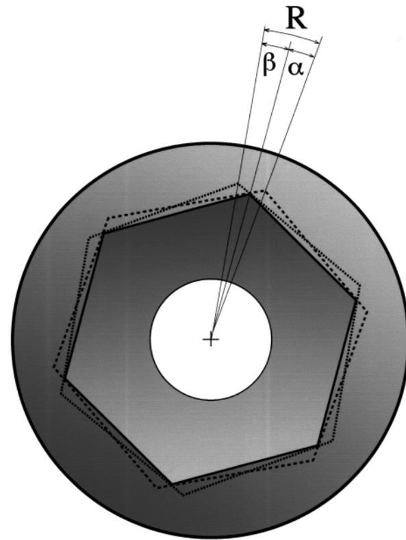
**Fig. 3.** Diagram illustrating rotational freedom ( $R$ ) between implant hexagonal extension and UCLA abutment counterpart.  $R$  represents difference between clockwise ( $\alpha$ ) and counterclockwise ( $\beta$ ) rotation of needle pointer attached to UCLA abutment collar.
