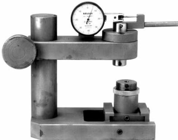
**Fig. 2.** Custom-made apparatus used to assess rotational freedom at implant-abutment interface.
