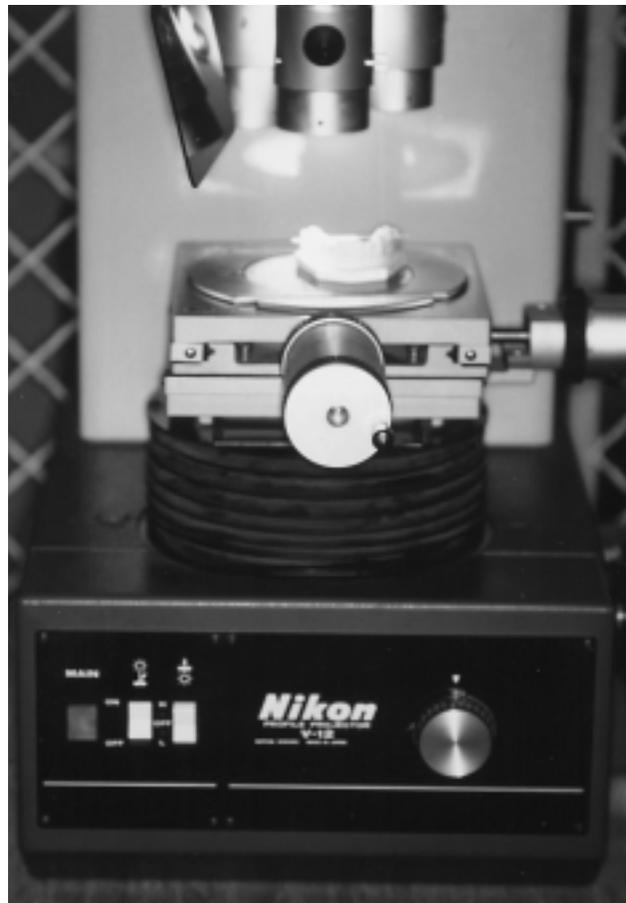
Fig. 3. Nikon Profile projector and master cast specimen.
