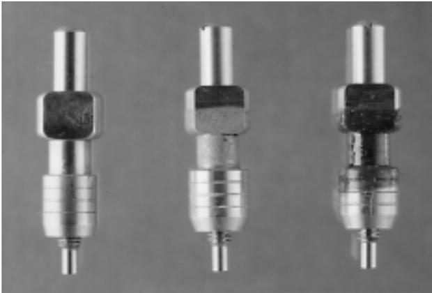
Fig. 2. From left to right, transfer copings as-received, sand-blasted, and coated with impression adhesive.
