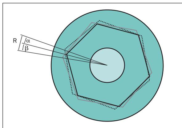
**Fig 3** Diagram illustrating rotational freedom (R) between the hexagonal extension of the implant and Procera abutment counterpart. R represents difference between clockwise ( $\alpha$ ) and counterclockwise ( $\beta$ ) rotation of the needle pointer attached to the Procera abutment collar.
